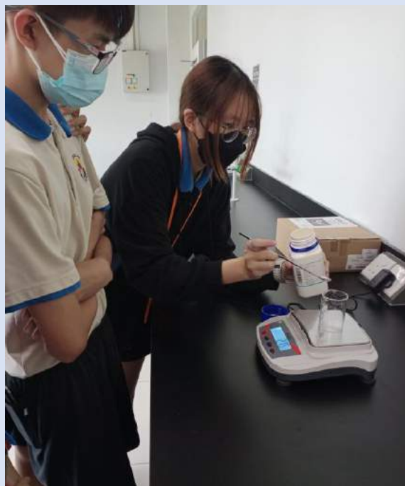
Students measure the sodium chloride using a weighing balance.
